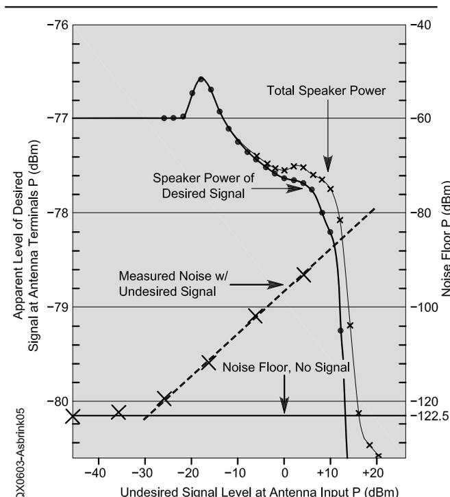
Figure 5 — The loudspeaker output of an FT-1000D with a 14.178 MHz on-channel signal at a level of -77 dBm (10 dB below the on-channel CP1) as a function of the off-channel signal level at 14.158 MHz. The dots are the on-channel signal level measured at 5 Hz bandwidth, the small crosses are the power (10 Hz to 24 kHz) and the big crosses are the power measured without the on-channel signal.
