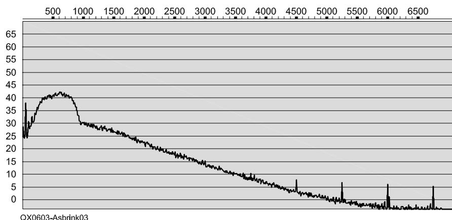
Figure 3 — The loudspeaker output from an FT-1000D with a noise source at the antenna input. All settings are identical to those of Figure 1.
